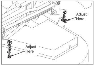
Figure 41. Hanger Chain Adjustment
